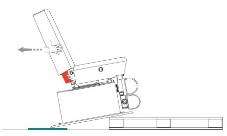
2. Grip the two armrest mountings on the right/left of the back section as shown. Pull the treatment chair off the pallet in the direction indicated by the arrow until the floor plate is sitting on the protective mat.
