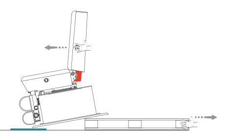
4. Grip the two armrest mountings on the right/left of the back section as shown. Lift the treatment chair and have a second person pull out the pallet from underneath.
