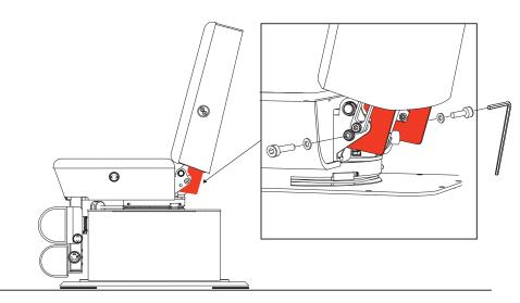
Before starting to remove the transport lock, protect the wood cover of the lift cladding and the floor plate of the treatment chair. Use a socket head wrench to loosen the hexagon socket screw on the right/left and remove with the corresponding washer.
