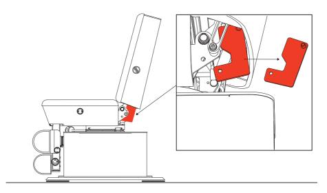
10. The transport lock can now be swung down and taken off with ease.
