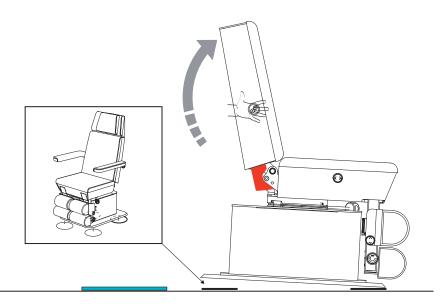
7 Grip the two armrest mountings on the right/left of the back section as shown. Lift the treatment chair and have a second person place two levelling pads under the floor plate.
