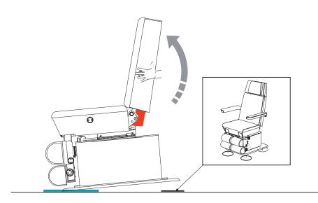
5. Grip the two armrest mountings on the right/left of the back section as shown. Lift the treatment chair and have a second person place two levelling pads under the floor plate.
