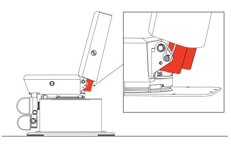
8. The two red transport locks must be removed before commissioning the treatment chair. Failure to do so may mean that the back section cannot be tilted, the drive and/or seat and back section may thereby be damaged.
