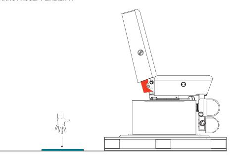
1. Before unloading the treatment chair, place a protective mat (e.g. foot mat) in front of the pallet to protect the floor.
