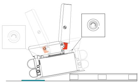
3 Turn the treatment chair by 180° so that the foot supports do not come into contact with the pallet when lowering. To do this, turn the hand wheel for rotation.
