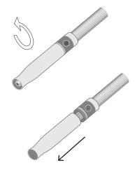
Carefully remove the sleeve by pressing against the metal cover of the chuck at the same time.
